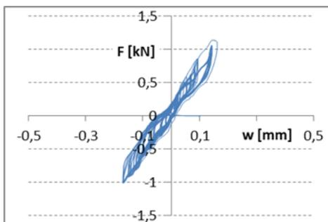
Fig. 18 - Hysteresis for load level 1 up to  $V = 1$  kN
