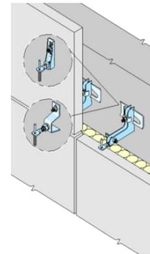
Fig. 6 – Example of bolted anchors
