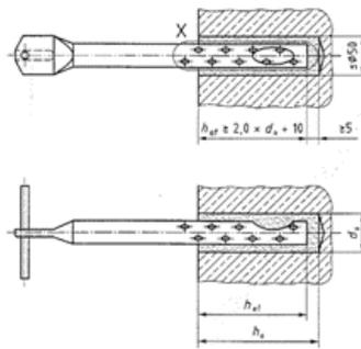
Fig. 5 – Example of cast-in anchors
