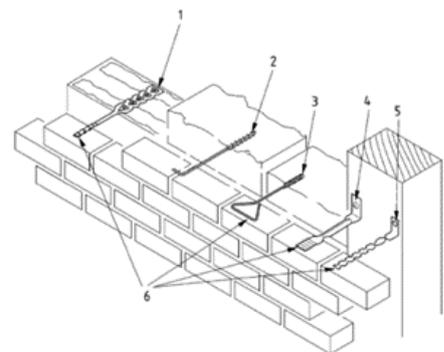
Fig. 3 – brick ties acc. to [1]
