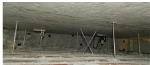
Fig. 21 - Wall ties after load level 1 up to  $V = 1$  kN
