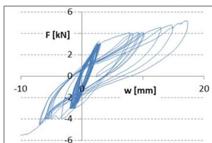
Fig. 20 - Hysteresis for load level 3 up to failure
