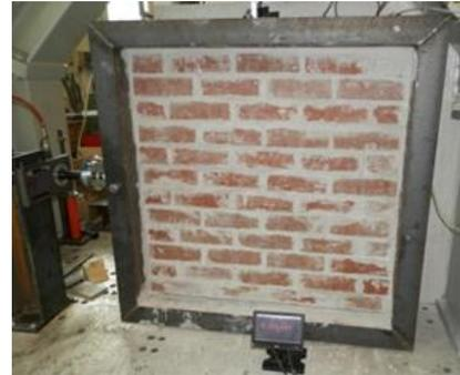
Fig. 17 - Meso-scale test setup of the brickwork support system
