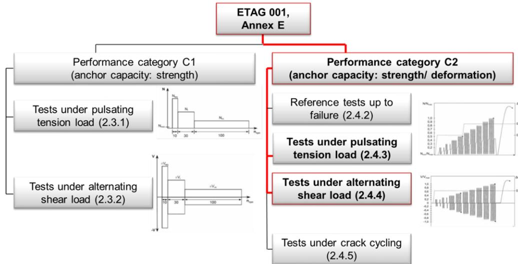
Fig. 15 - Test procedure according to [3]
