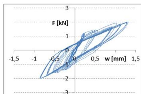
Fig. 19 - Hysteresis for load level 2 up to  $V = 2$  kN
