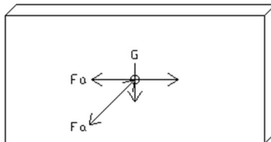
Fig. 10 – Load directions in earthquake design
