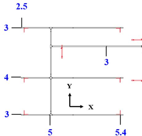
Fig. 15 – Case A max. displacement under JMA KOBE25%. (mm)
