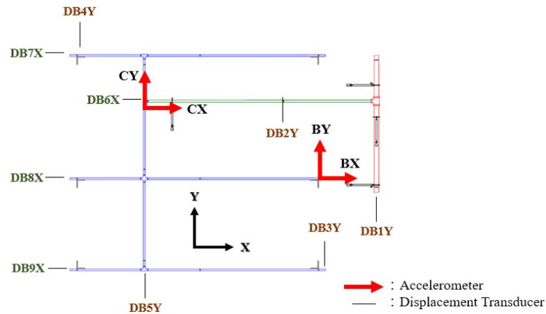
Fig. 13 – Accelerometer and displacement transducer configuration.
