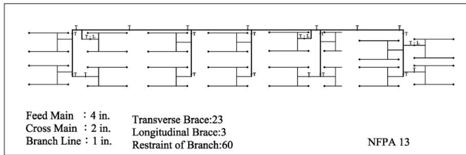
Fig. 2 – Configuration for NFPA13.
