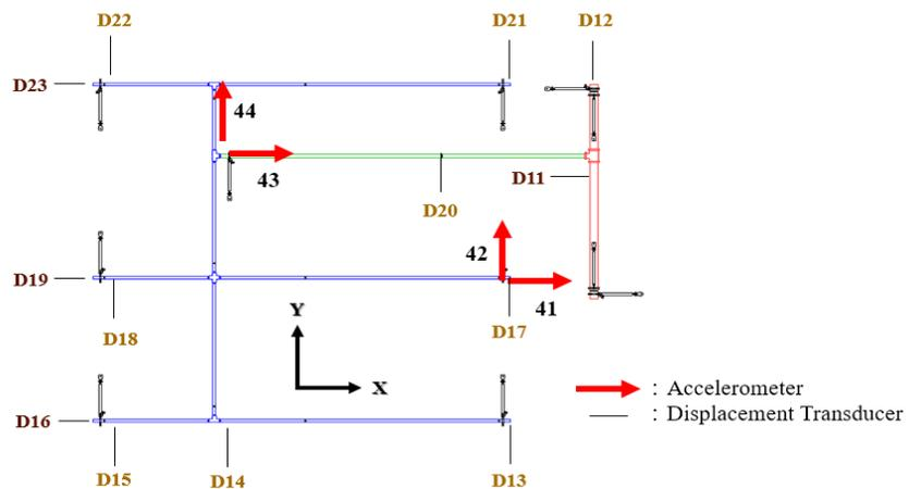
Fig. 8 – Accelerometer and displacement transducer configuration.
