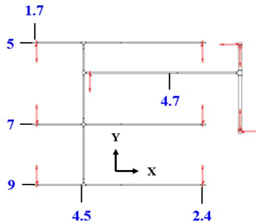
Fig. 10 – Case 1 max. displacement under JMA KOBE25%. (mm)
