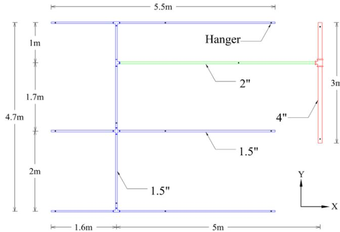
Fig. 6 – Piping system scale for shaking table test.
