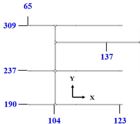
Fig. 16 – Case B max. displacement under JMA KOBE25%. (mm)
