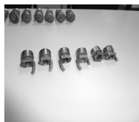
c. Sprinkler heads sheared off
