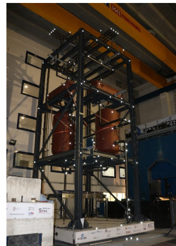
Fig. 2 – Marker of the vision system for the displacement measurement
