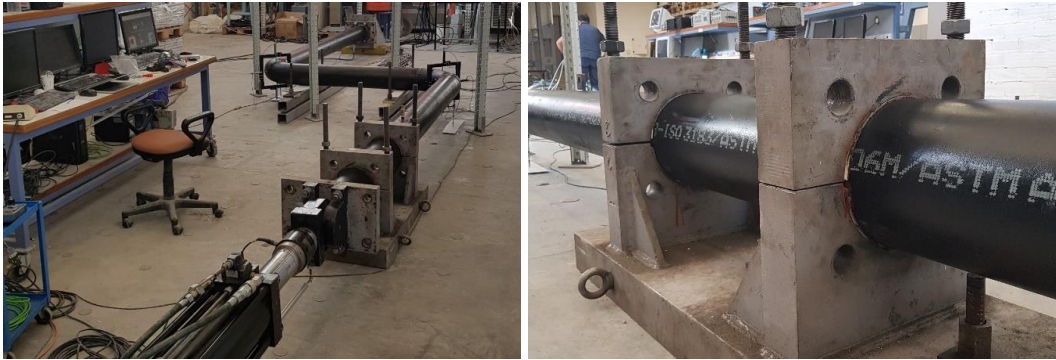
Fig. 4 – Physical substructure module (left) and the auxiliary restraint device (right).
