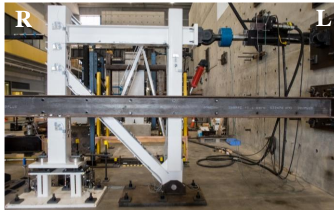
Fig. 7 – Assembled specimen of the centralised rocking test frame [9]
