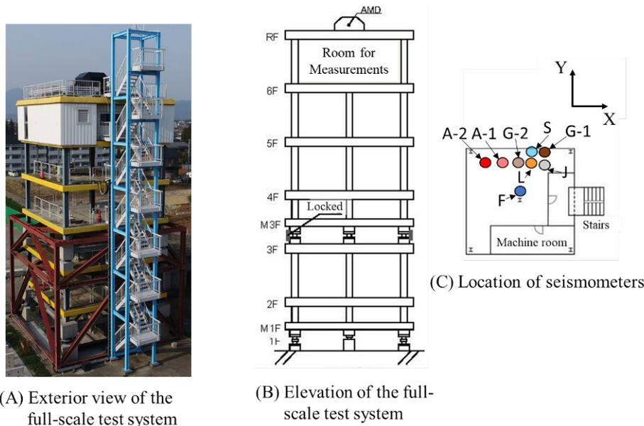
(A) Exterior view of the full-scale test system
