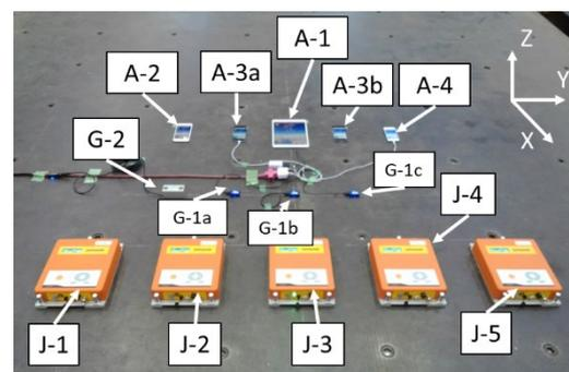
Photo 1 – Positions of measurement devices on the shaking table.
