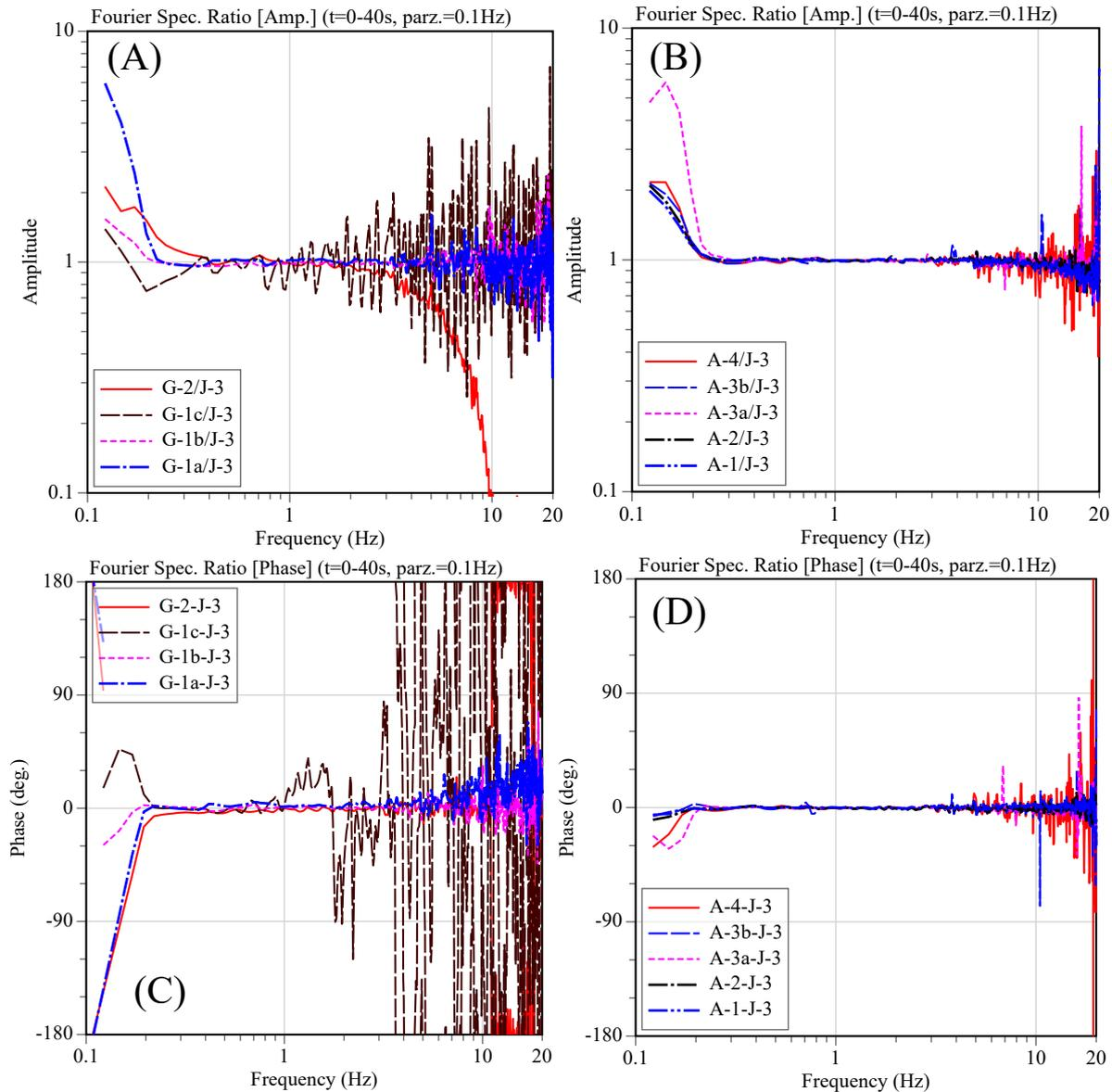
Fig. 1 – Comparison of measurement performance between measurement devices. A: amplitudes of G-1a, G-1b, G-1c, G-2, B: amplitudes of A-1, A-2, A-3a, A-3b, A-4, C: phases of G-1a, G-1b, G-1c, G-2, and D: phases of A-1, A-2, A-3a, A-3b, A-4.
