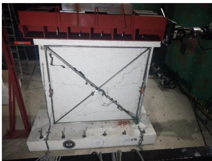
(b) Final cracking patterns of tested wall
