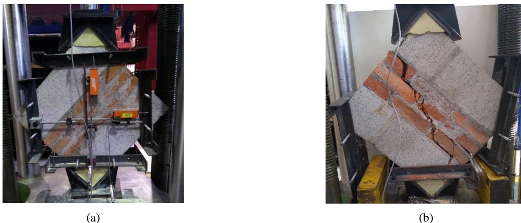
Fig. 4 – Combined masonry wallets arrangement, (a) instrumentation and (b) mode of failure
