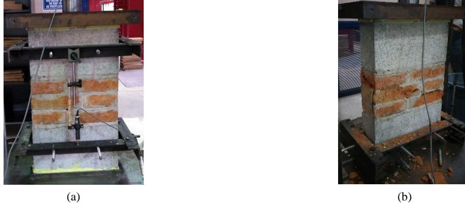
Fig. 3 – Combined masonry prism arrangements, (a) instrumentation and (b) mode of failure.
