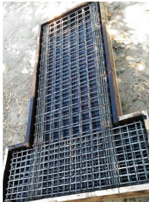
Fig. 4 – Reinforcement cage for specimen USW2
