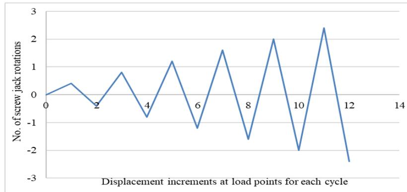
Fig. 9 –Displacement increments for each cycle as per the screw jack rotations
