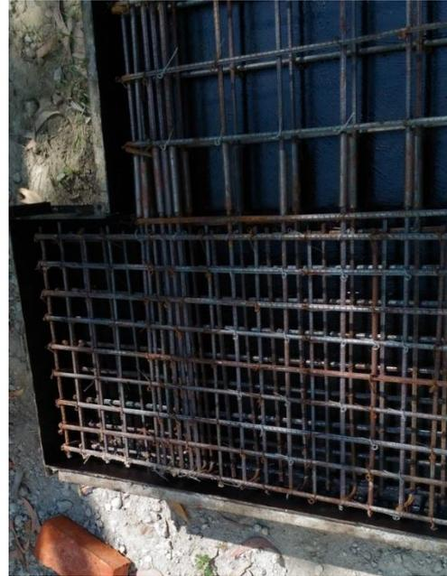
Fig. 6 – Reinforcement cage for specimen USW4
