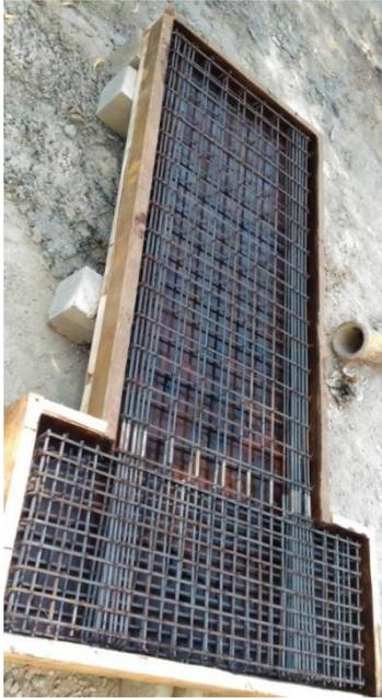
Fig. 5 – Reinforcement cage for specimen USW3
