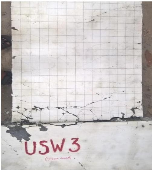
Fig. 17 –Crack Pattern for Specimen USW3
