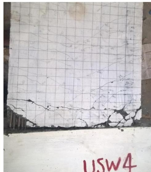
Fig. 18 –Crack Pattern for specimen USW
