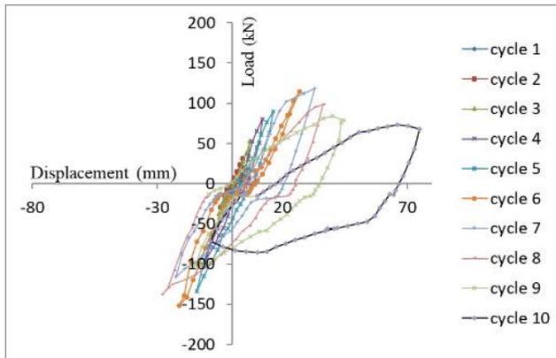
Fig. 12 –Load- displacement hysteresis curve of USW3
