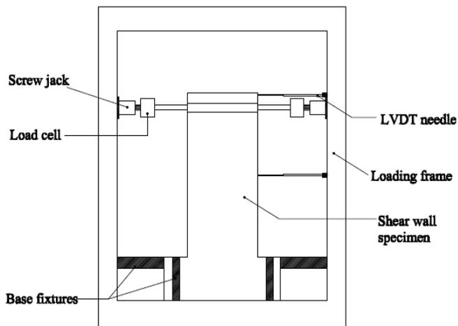
Fig. 7 – Schematic diagram of Experimental setup
