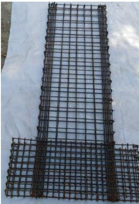
Fig. 3 – Reinforcement cage for specimen without collars (USW1)
