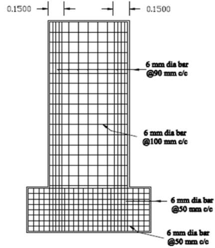
Fig. 2 – Reinforcement details of specimen
