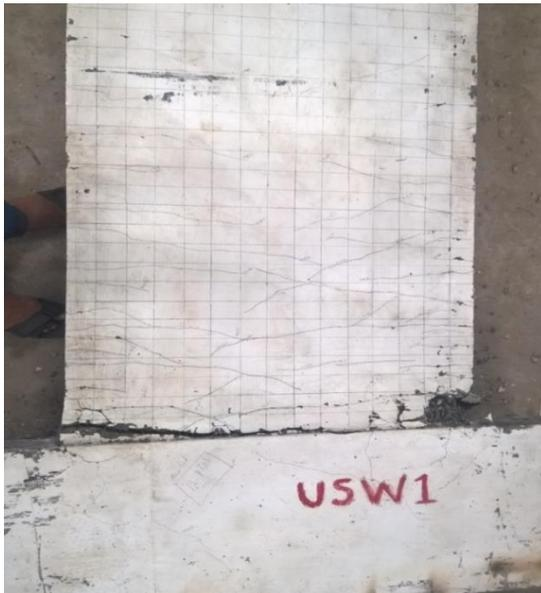
Fig. 15 –Crack Pattern for specimen USW1
