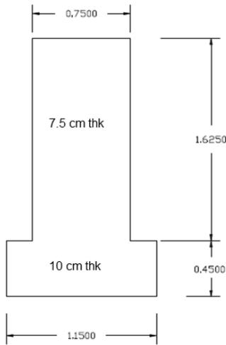
Fig. 1 – Specimen dimensions
