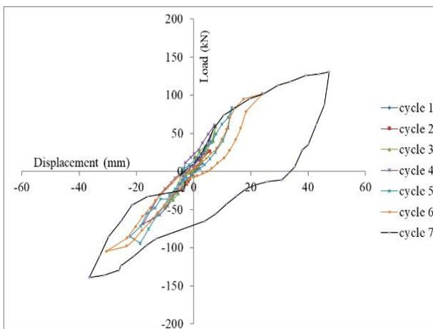
Fig. 10 –Load- displacement hysteresis curve of USW1
