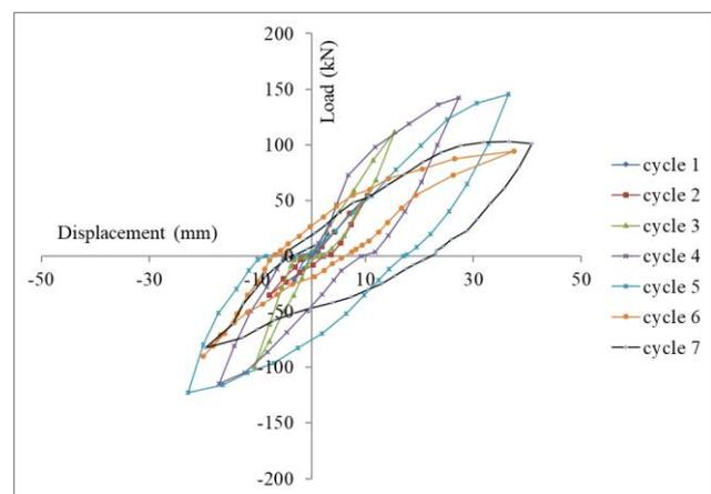
Fig. 11 –Load- displacement hysteresis curve of USW2
