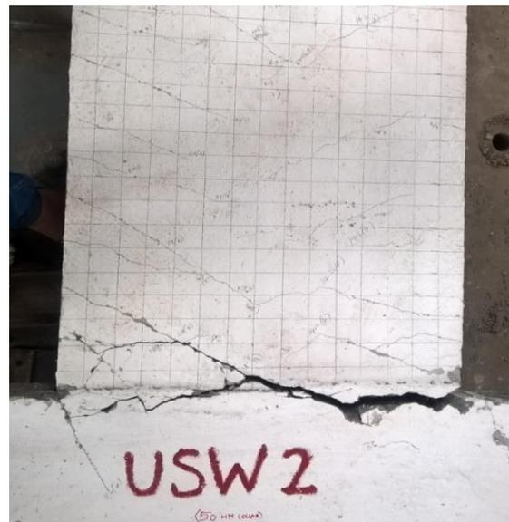
Fig. 16 –Crack Pattern for specimen USW2
