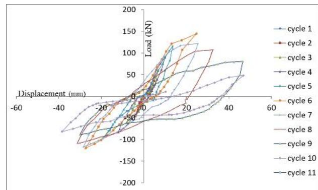
Fig. 13 –Load- displacement hysteresis curve of USW4
