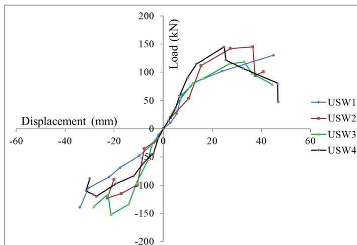
Fig. 14 –Load- displacement envelope curve for tested specimens
