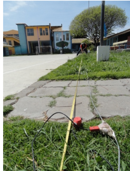
(b) ReMi seismic survey
