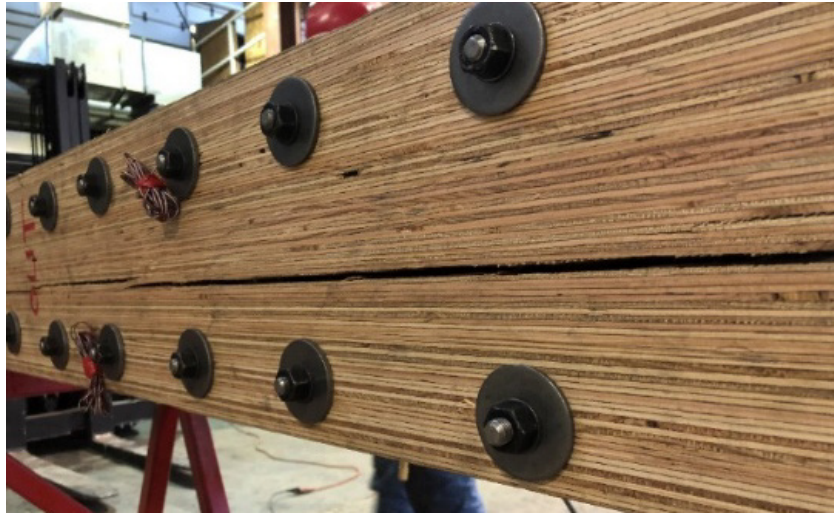
Fig. 12 – MPP split resulting from strong axis steel core buckling of specimen 6
