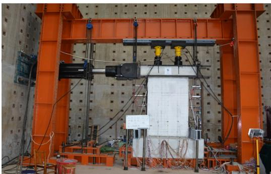
Fig. 4 – Loading apparatus
