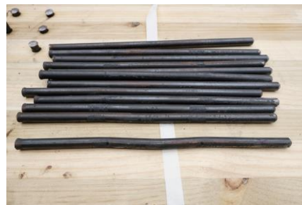
Fig. 8 – Dowels' bending in S-D specimen
