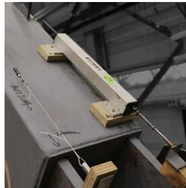
Fig. 6 – The linear-motion potentiometer for measuring BRB deformation
