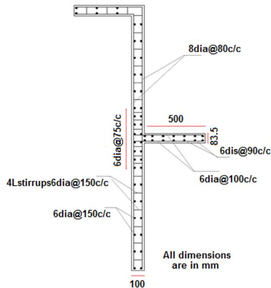
Fig.3 - Reinforcement details of sub-assembly unit
