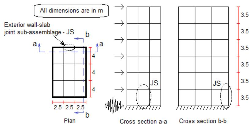
Fig. 1 – Details of the prototype building
