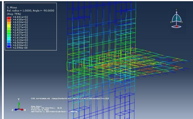
Fig.11 (c) - Von Mises stress at P2 joint
