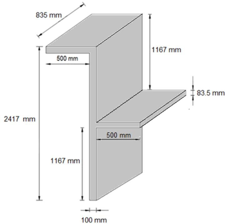
Fig. 2 - Geometry of sub-assembly unit
