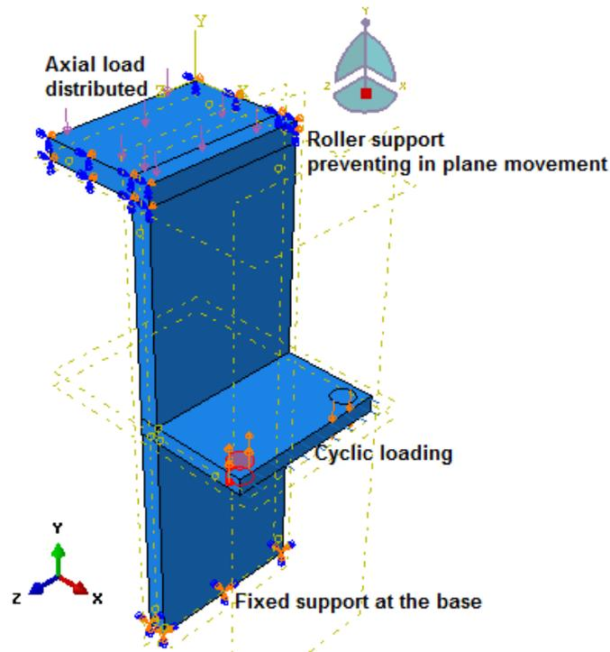
Fig. 9 - Loading and boundary conditions
