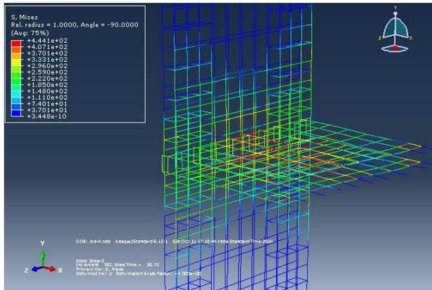
Fig.11 (b) - Von Mises stress at P1 joint
