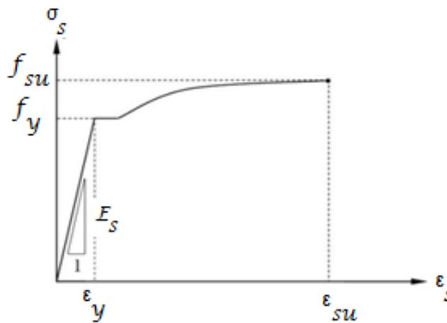
Fig. 5 - Stress strain characteristics of steel
