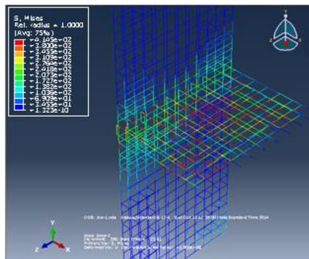
Fig.11 (a) - Von Mises stress at C joint
