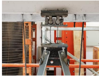
Fig. 3 – Energy dissipation device of EPSCF
