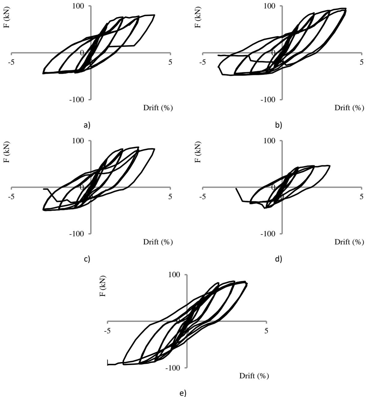
Fig. 5 – Hysteretic force-displacement response
