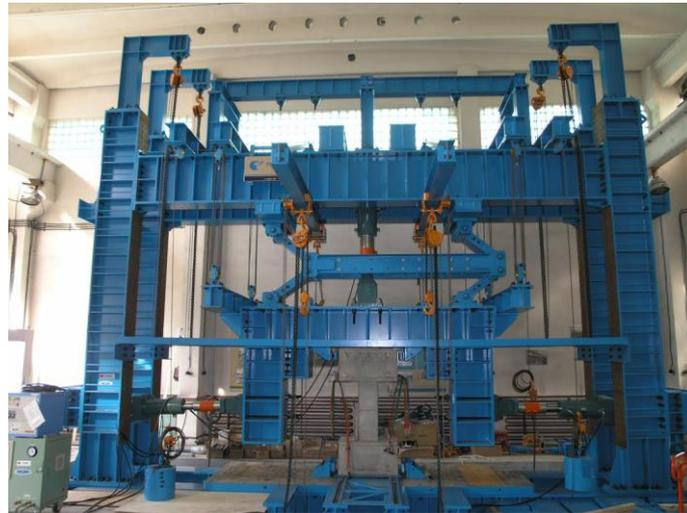
Fig. 4 – Reaction frame [1]
