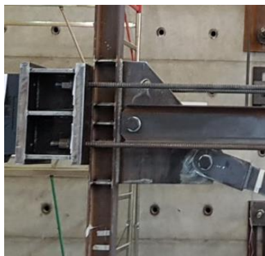
Figure 3 - Steel connection plate of the CSB with the pendular frame: (a) picture, (b) geometric details.
