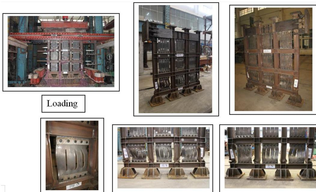
Fig.5 Failure state of specimen MSW-3
