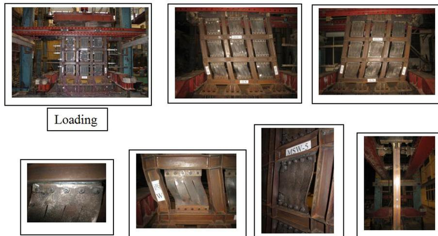
Fig.7 Failure state of specimen MSW-5
