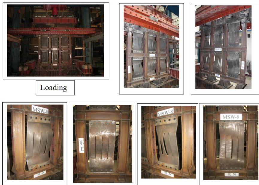
Fig.10 Failure state of specimen MSW-8
