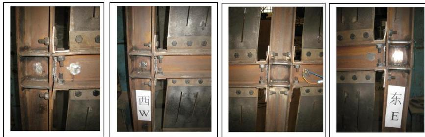
Fig.8 Failure state of specimen MSW-6
