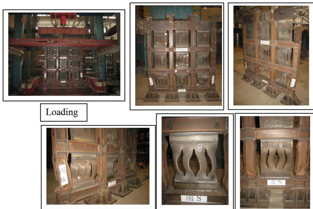
Fig.6 Failure state of specimen MSW-4
