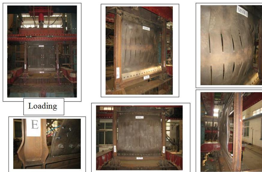
Fig.3 Failure state of specimen MSW-1
