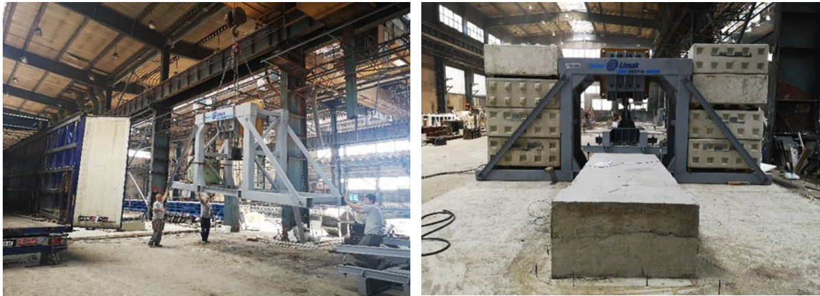
Fig. 14 Mounting of the Hydraulic Jack with supporting structure and additional concrete blocks
