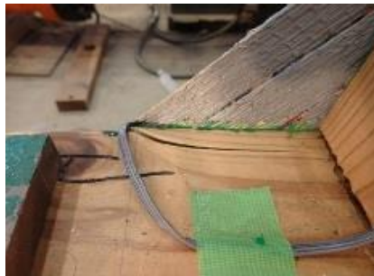
(b) Splitting the specimen at 1/8 rad.
