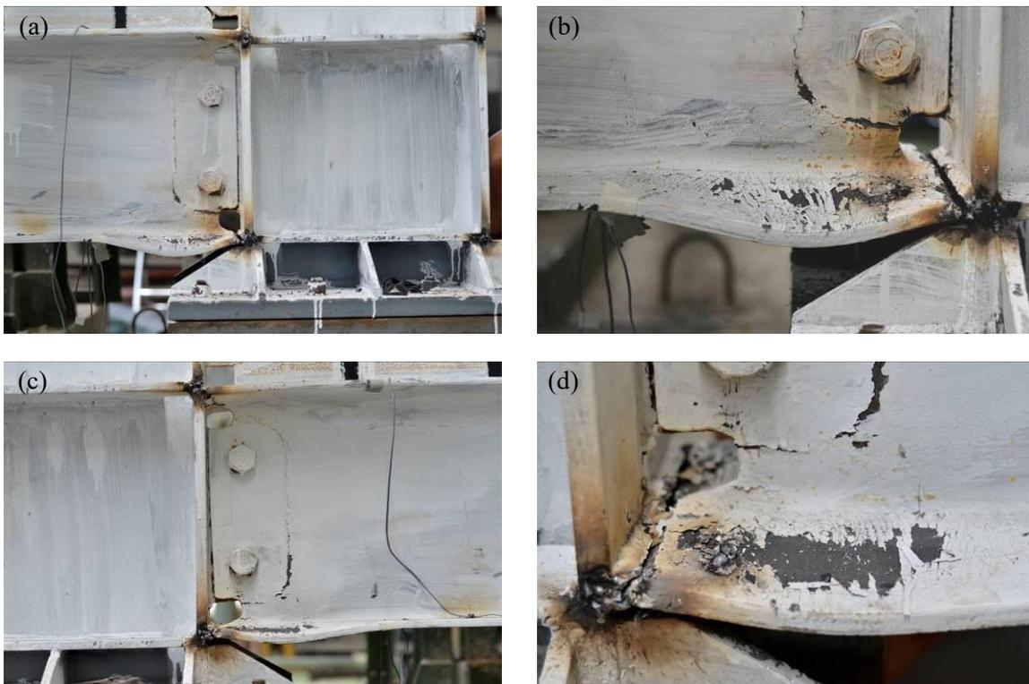
Fig. 7 – Final Condition of WUF-W Specimen at the Bottom HBE-to-VBE Connections: (a) East Connection, South View; (b) Detail of (a); (c) West Connection, South View; (d) Detail of (c)
