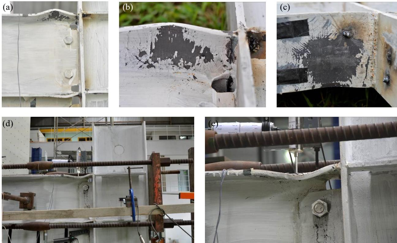
Fig. 8 – Final Condition of WUF-W Specimen at the Top HBE-to-VBE Connections: (a) East Connection, South View; (b) and (c) Detail of (a); (d) West Connection, North View; (e) Detail of (d)
