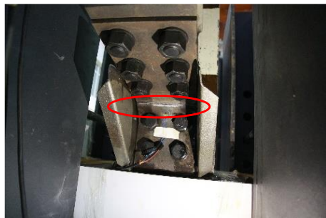
(e) Bottom angle ruptured at Section NE (5, \Delta = 451 mm, F = 348 kN)
