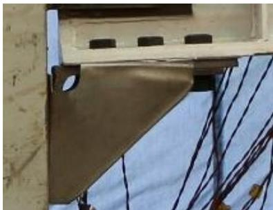
(c) Rib stiffener ruptured (B,  $\theta = 0.045$  rad)
