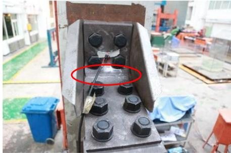
(c) Top angle ruptured at Section SA
