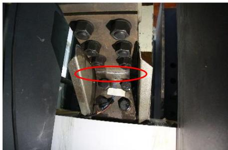
(e) Bottom angle ruptured at Section NE
