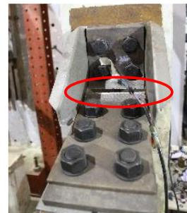
(f) Top angle ruptured at Section NA
