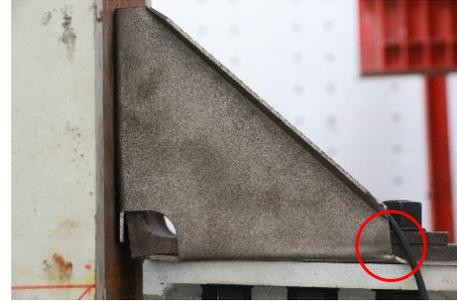
(b) Tension rib stiffeners began to rupture
