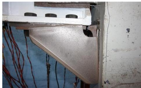
(d) Angle steel under south beam ruptured (C,  $\theta = 0.033$  rad)
