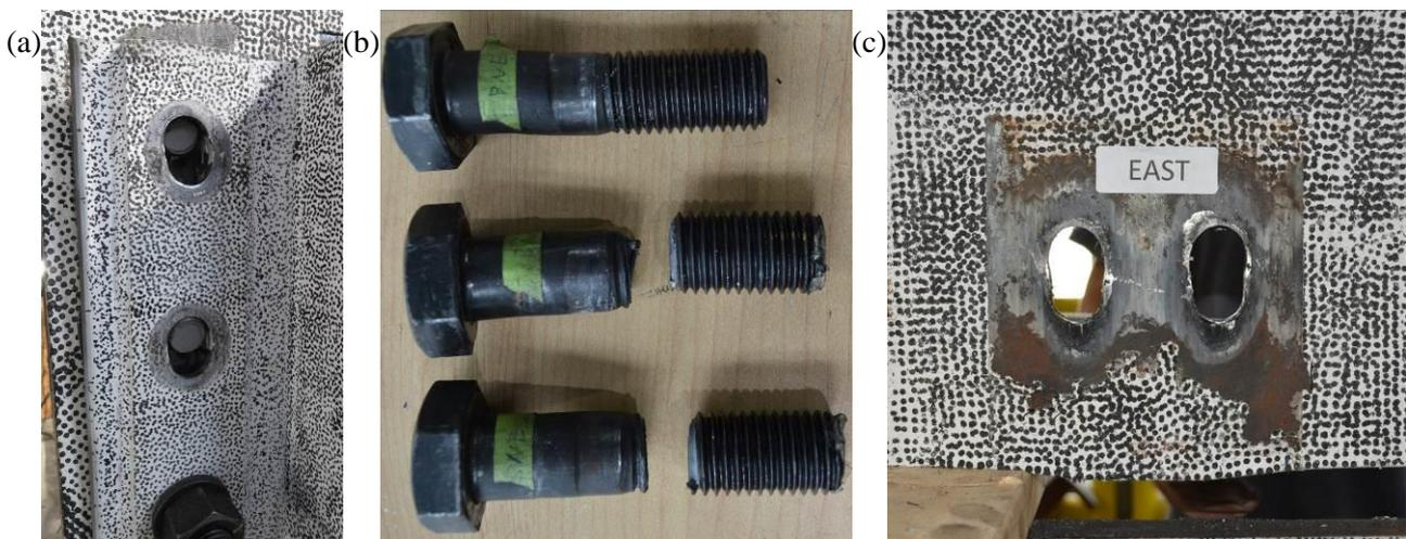
Fig. 6 – Observed damage in flange angle connection (Specimen C360-P): (a) bearing deformations in fuse plate and bolt fracture, (b) bolt fracture, (c) block shear failure in web of brace
