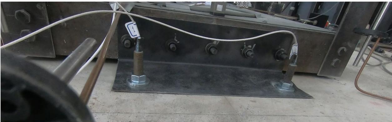
Fig.7. Uplift of NEMO attached with the long-thin angles during Morgan Hill motion.
