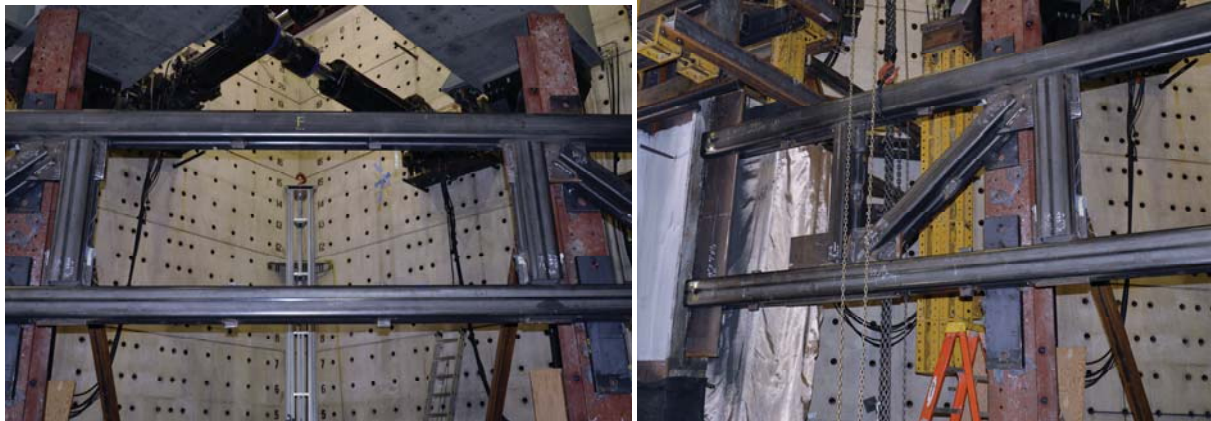
Fig. 4 – Double-HSS truss members for special truss moment frames
