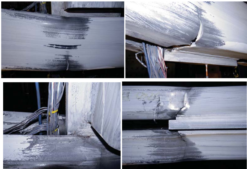
Fig. 11 – Members in the special segment at the end of testing
