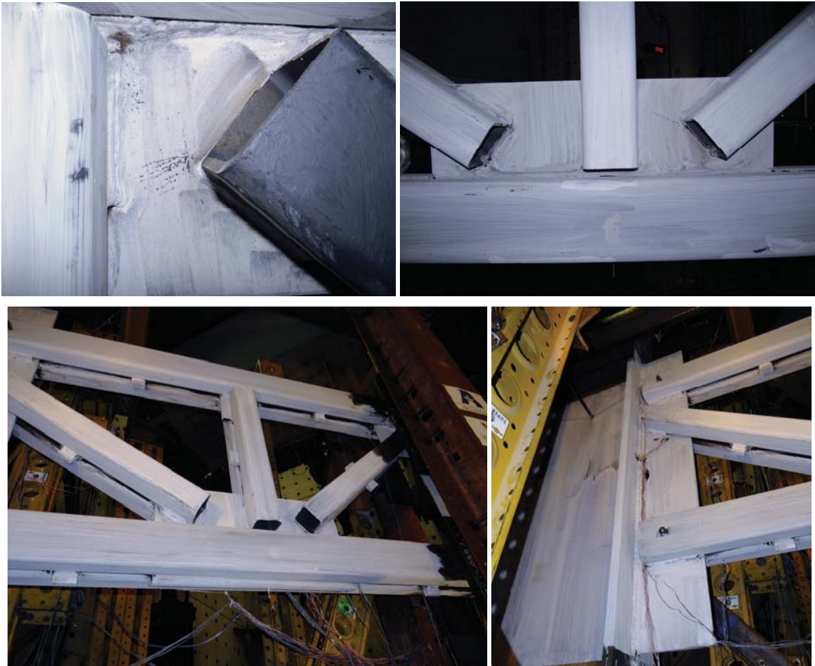
Fig. 12 – Members outside of the special segment at the end of testing
