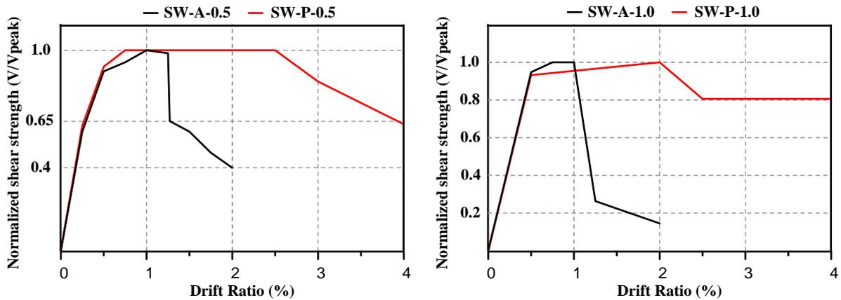
Fig.6– Normalized shear strength backbone curves of 0.5 and 1.0 aspect ratio walls.
