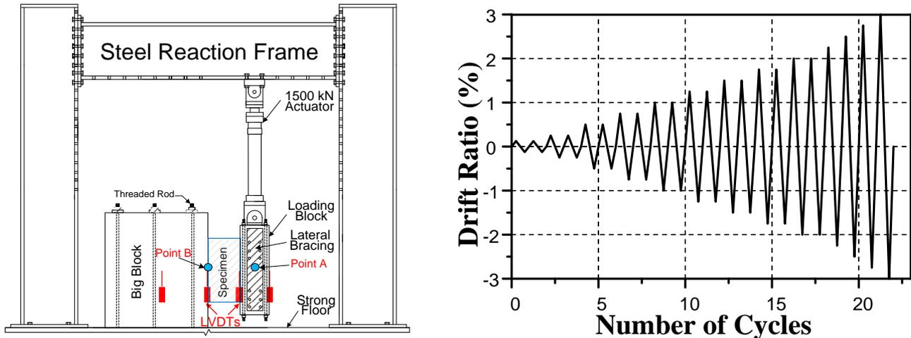
Fig. 2 – Test setup and loading protocol.
