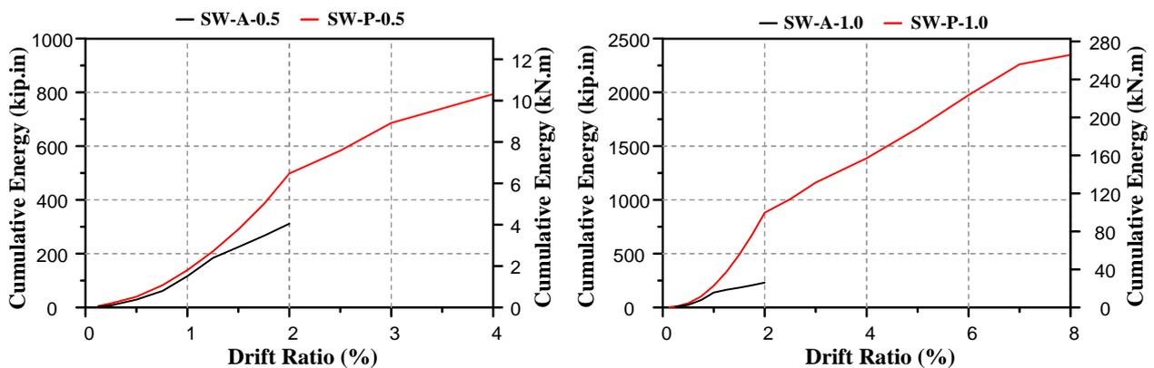
Fig.7– Cumulative energy curves of 0.5 and 1.0 aspect ratio walls.
