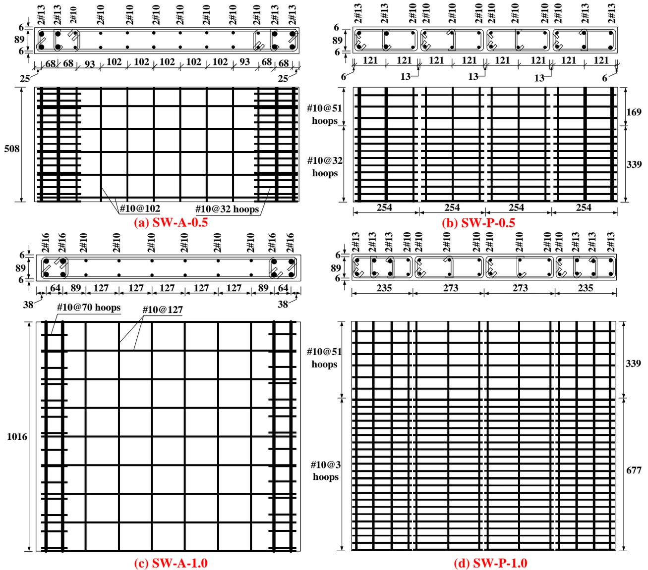
Fig. 1 – Specimen reinforcement details (units: millimeter). All bars sizes are in metric size.
