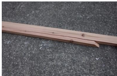
(e) W-side stud splitting when dismantling
