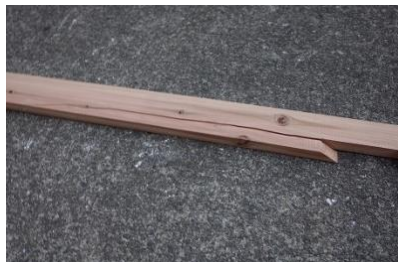
(e) W-side stud splitting when dismantling
