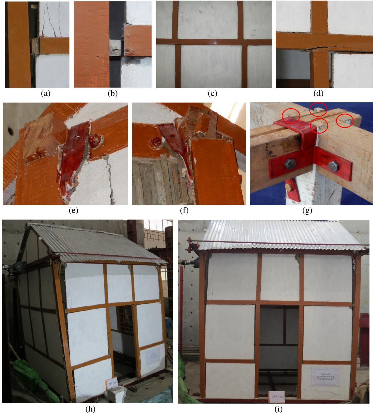
Fig. 7 – Damage observed in various components of the house during quasi-static testing: (a) Pullout of Joint D, (b) Pullout of Joint E, (c) Sliding movement of vertical stud and Ikra panels, (d) Tearing of top joint of doorpost, (e) Damage to top main post joint (Joint C'), (f) Hook-type steel flat in Joint C', (g) Small thickness of main post unable to prevent damage at Joint C', (h) Out-of-plane movement of transverse wall under lateral loads, and (i) Damage in the wall with door opening after 240 mm displacement
