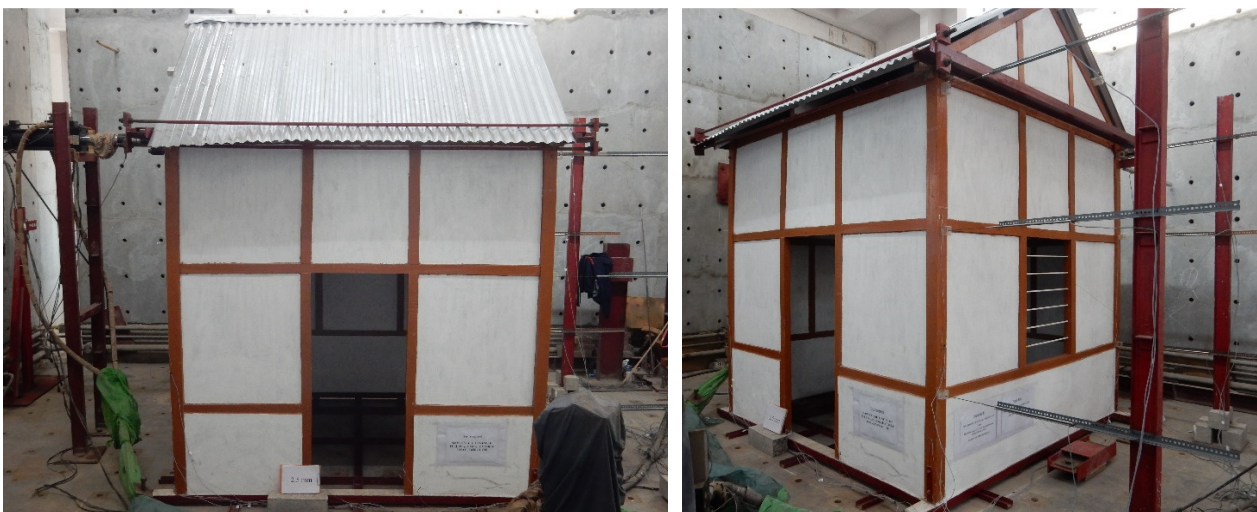
Fig. 2 – Full-scale Assam-type house specimen tested under quasi-static cyclic loading
