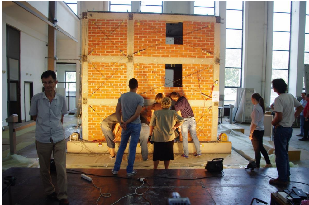
Fig. 2 – Series 1 model building during testing on the shaking table
