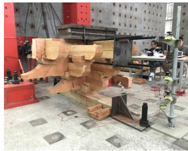
Fig. 4 –Horizontal loading setup
