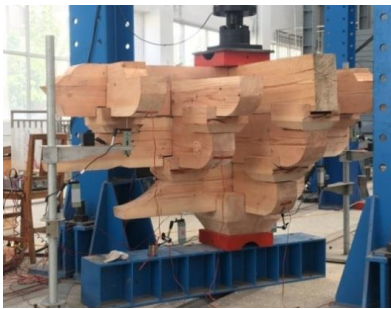
Fig. 3 –Vertical loading setup
