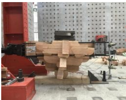
(c) The overall tilt of the Dougong
