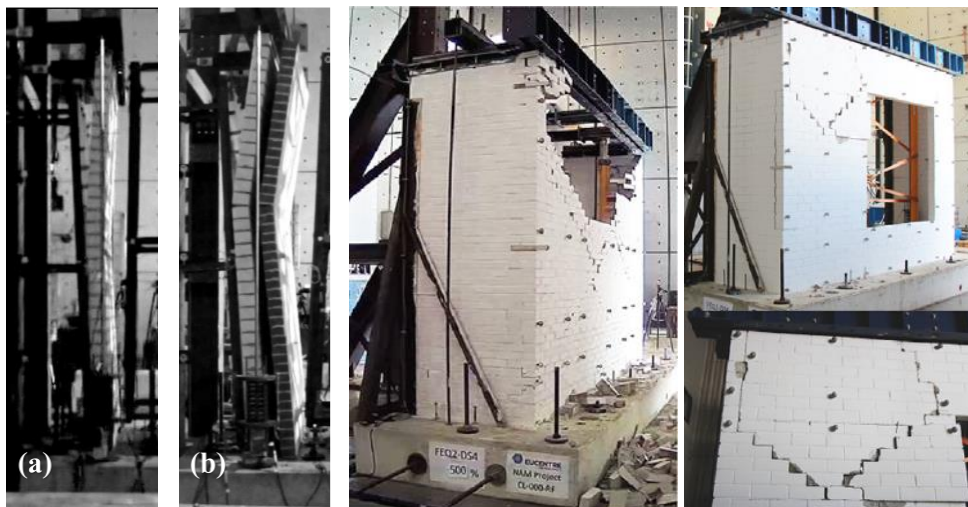
Fig. 7 - Picture of collapses of the one-way- and two-way bending specimens subjected to out-of-plane shaking table tests
