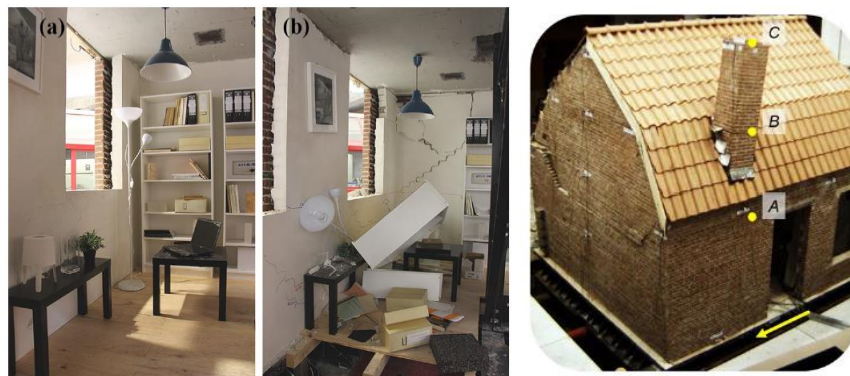
Fig. 9 – Pictures of LNEC-B1 and -B3 specimens, damage to nonstructural components
