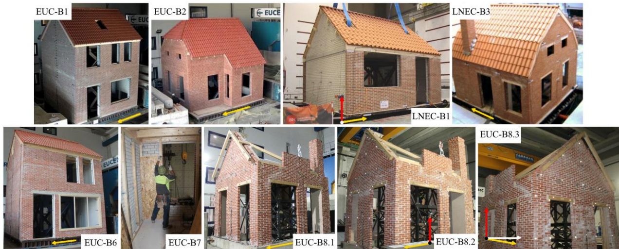
Fig. 8 - Pictures of full-scale building specimens tested on shake tables of EUCENTRE and LNEC
