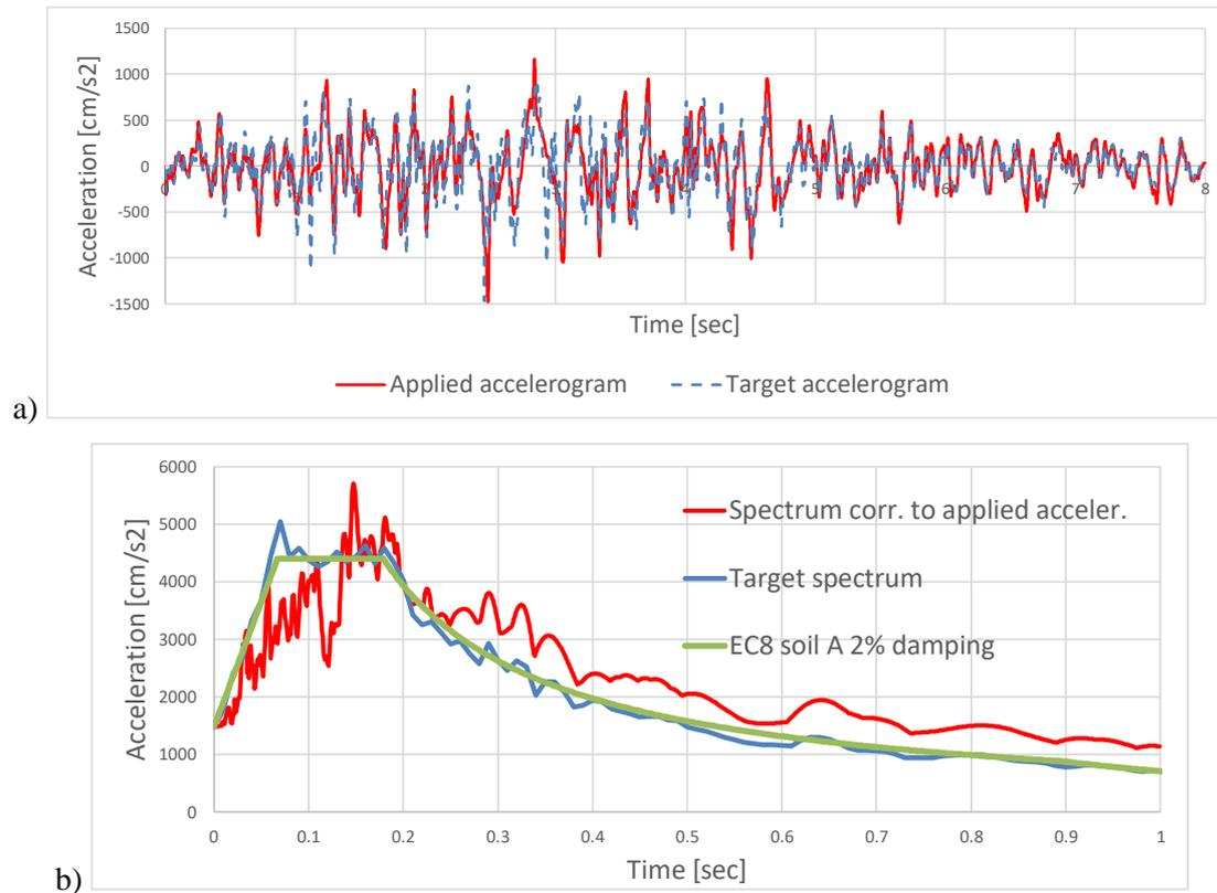
Fig. 4 – Seismic excitation: a) target and applied accelerogram, b) corresponding acceleration spectra for PGA = 1,5 g (Note: The time axis is scaled considering time scale factor from Table 1).
