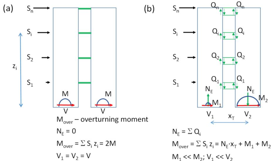
Fig. 2 – Resisting mechanisms: a) cantilever walls (very weak coupling), b) coupled walls (significant coupling of wall piers)
