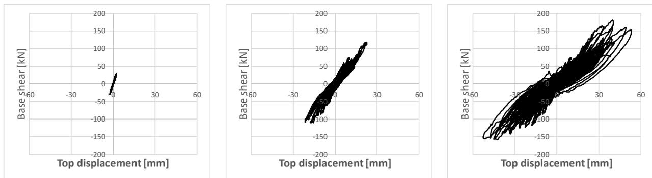
Fig. 10 – Hysteretic response at three different stages of testing: a) after R010, b) after R060(2) and c) after the last test R150(2)
