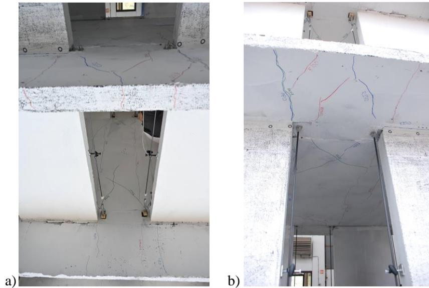
Fig. 6 – Cracks were formed at a) the top and b) at the bottom surfaces of the slabs, all over their width between two rows of wall piers
