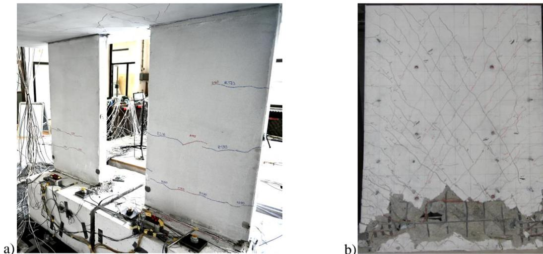
Fig. 7 - a) Cracks, which were observed in the wall piers,
