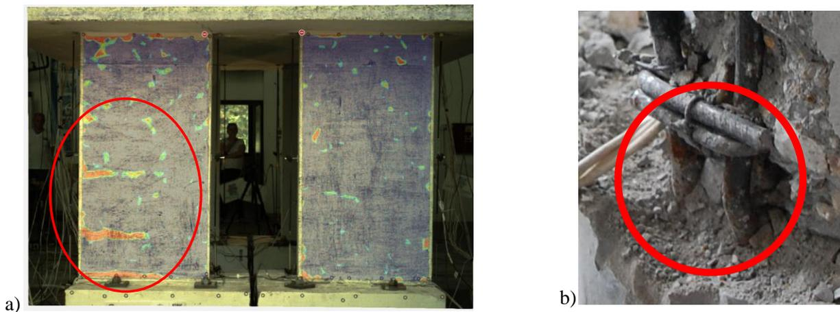
Fig. 8 – a) Response of two piers was considerably different, b) Buckling of the longitudinal bars was observed in the outer edge of one pier
