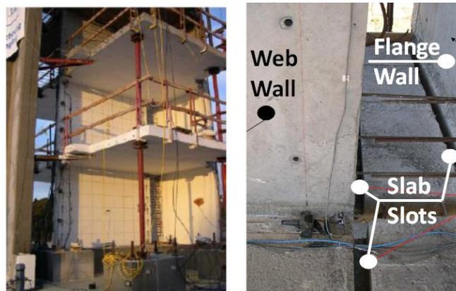
Fig. 1 – Cantilever RC wall tested at shake table at UCSD:
