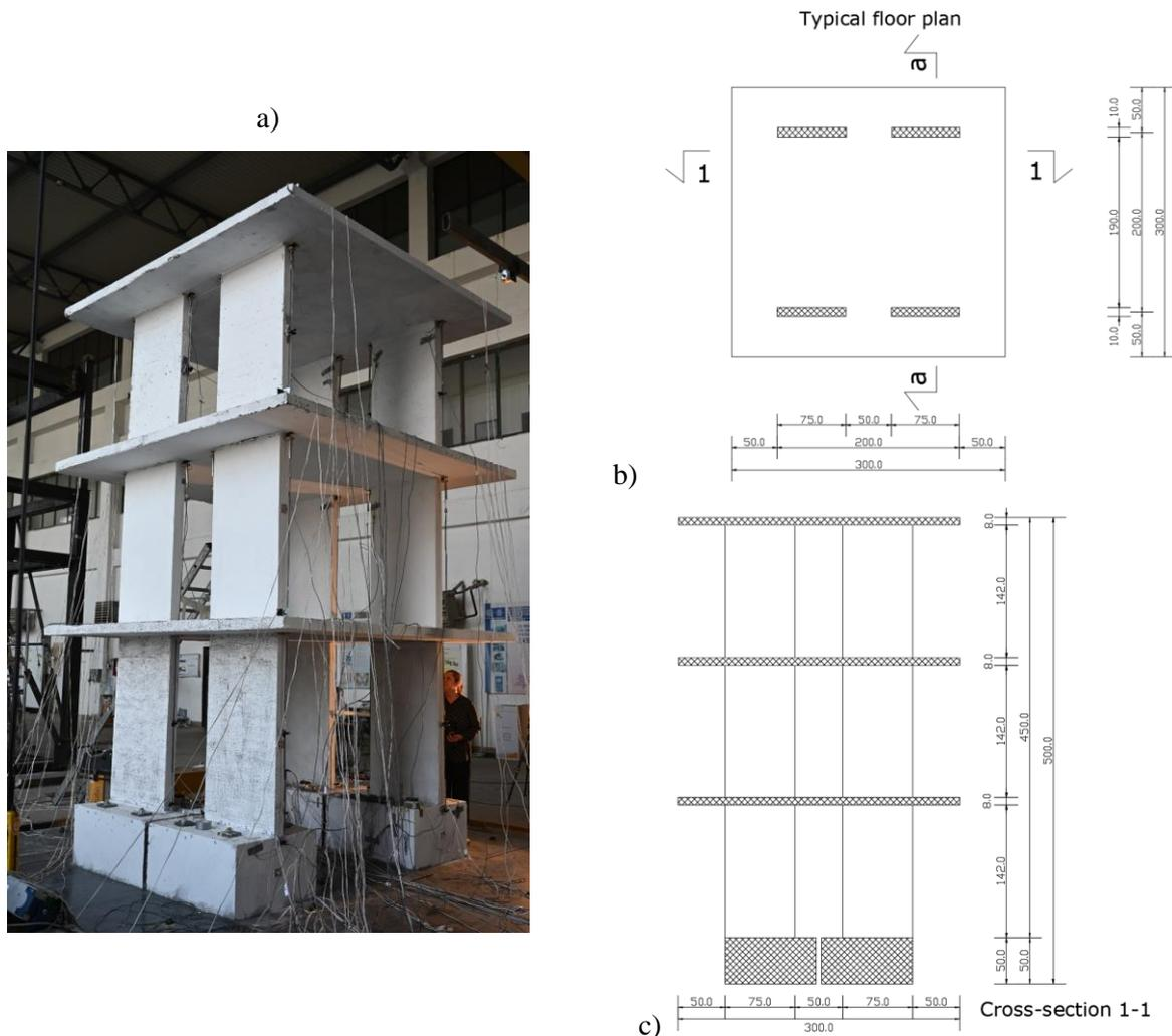
Fig. 3 – The specimen and its geometry: a) the appearance, b) floor plan, c) side view
