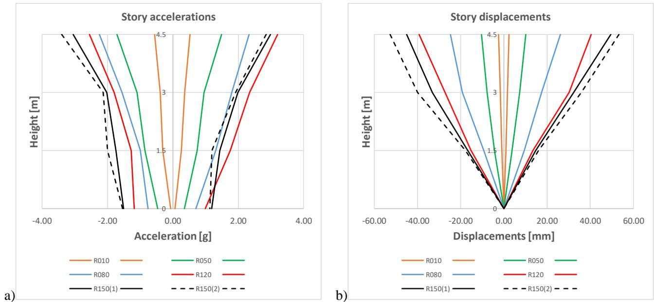
Fig. 9 – Envelopes of a) horizontal story accelerations, b) horizontal story displacements in the direction of excitation
