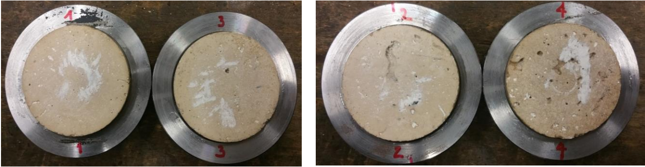
Fig. 8 – Minimal wear on the contact surfaces after the friction tests
