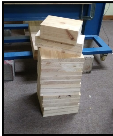
Fig. 2 – Five plies CLT elements [6]
