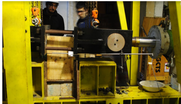
Fig. 4 –Assembly for cyclic tests of wall joints on its own plain (P) [6]
