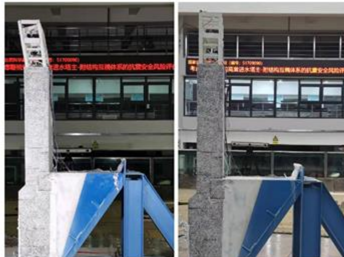
Fig. 13 – Residual deformation of the model at the end of the experiment
