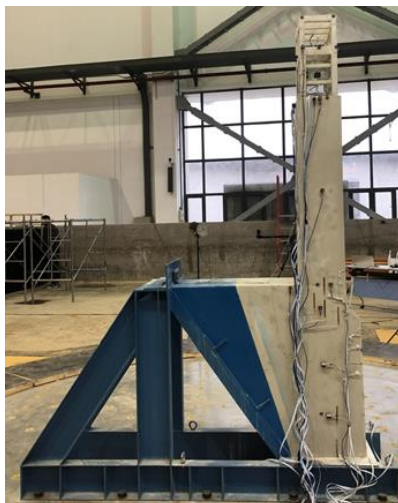
Fig. 4-The arrangement of acceleration sensors and strain gages
