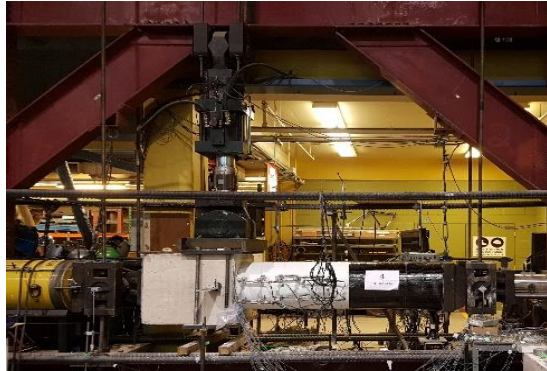
Fig. 2 – (a) CTF test set-up; and (b) Lateral loading protocol
