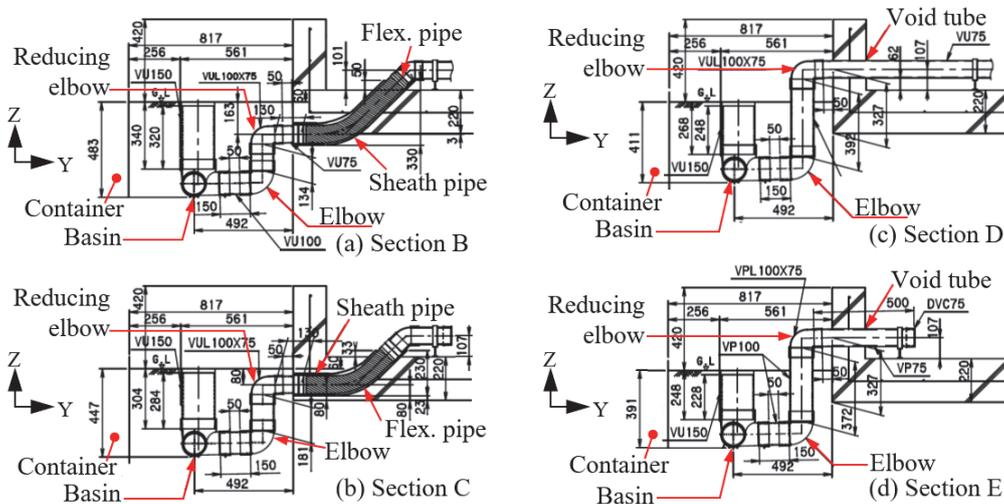
Fig. 4 – Details of Sections B to E
