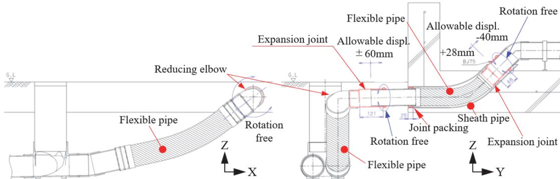
Fig. 3 – Details of Section A
