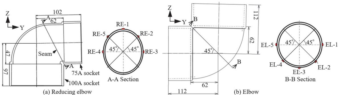
Fig. 6 – Locations of strain gages around elbow portions
