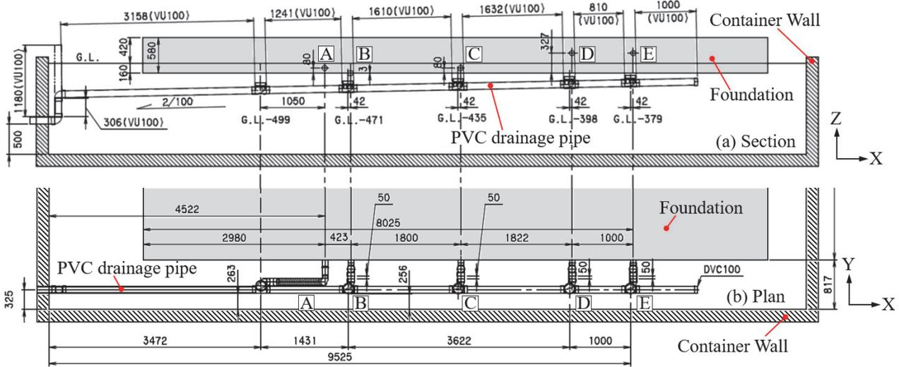
Fig. 2 – Test setup (shaking table test)
