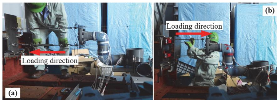
Fig. 18 – Test setup of static loading test in each direction
