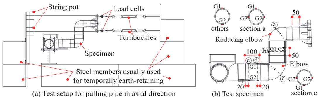
Fig. 17 – Dimensions of specimen and gage locations for static loading test
