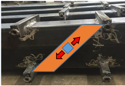
i) Inside type of diaphragm
