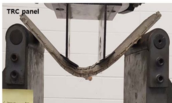
Fig. 3. Flexural test of TRC panel
