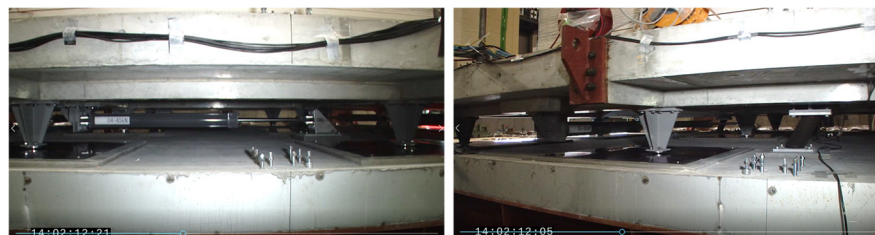
(2) Relative displacement in the base-isolation layer while subjected to JMA-Kobe 100 %
