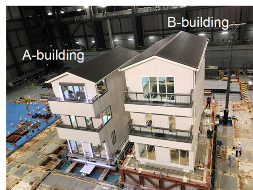
(2) Completion of setups in E-Defense
