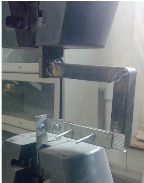
(a) Test along long leg of ceiling angle
