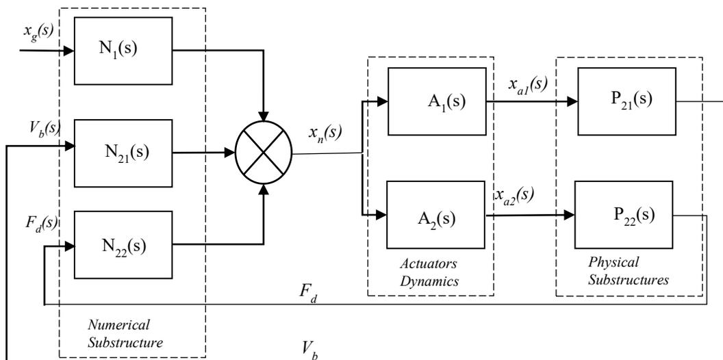
Fig.3 - The RTHS Feedback Loop for a Seismically Excited Base Isolated Building
