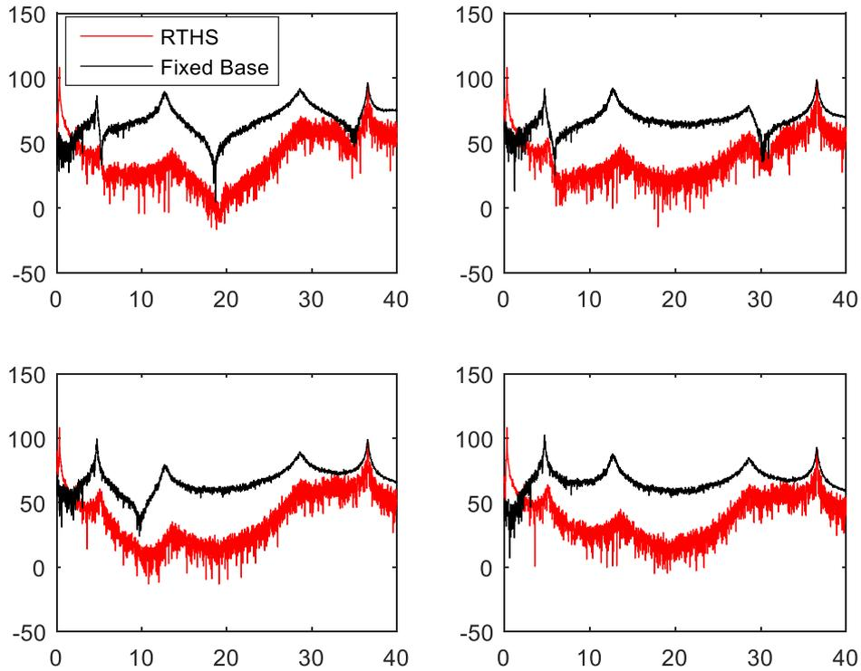
Fig. 7 Experimentally Determined Transfer Functions of Absolute Story Acceleration to Ground Acceleration for Fixed-Base(black) and Base Isolated (red) 4-Story Buildings.
