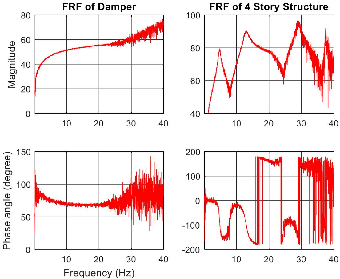
Fig.4 Transfer function of the viscous damper (left) and 4-story structure (right)
