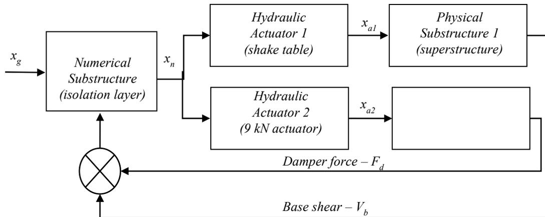
Fig.1 - Feedback Loop Block Diagram for RTHS
