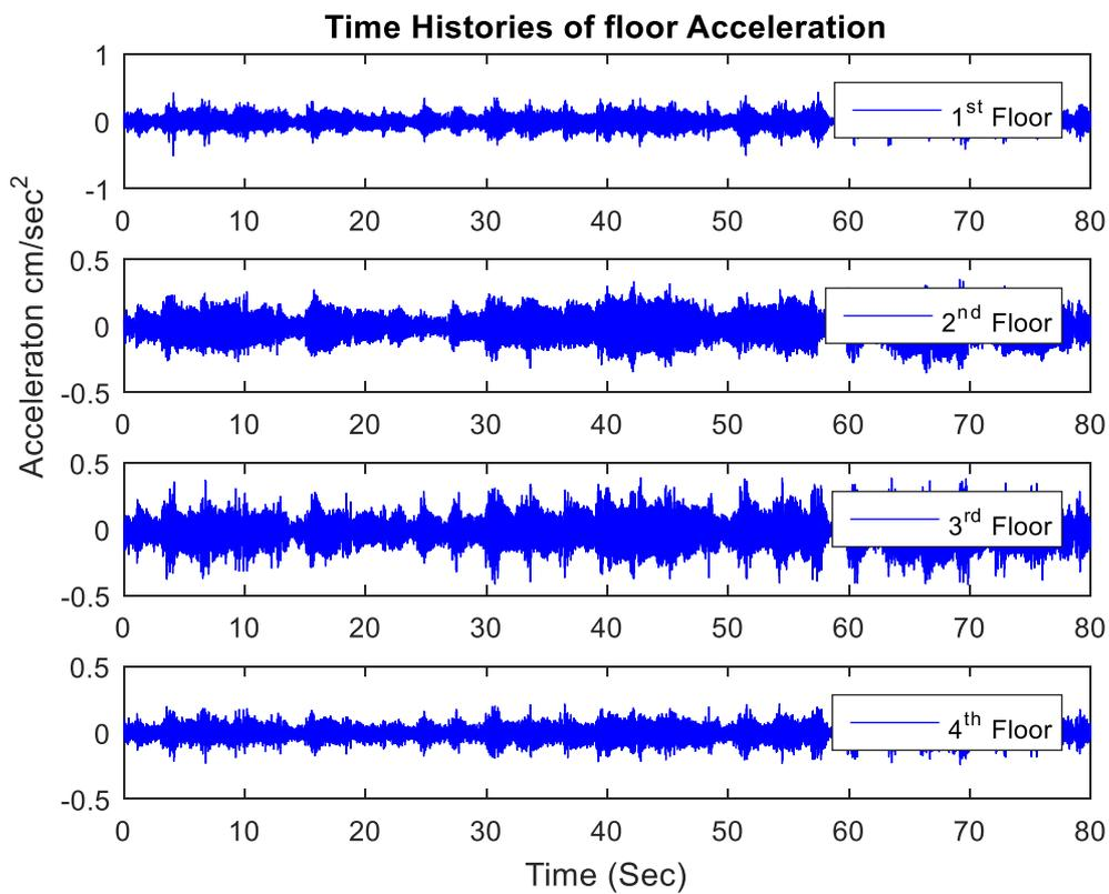
Fig. 8 Time Histories of Floor Acceleration on Base Isolated Superstructure.
