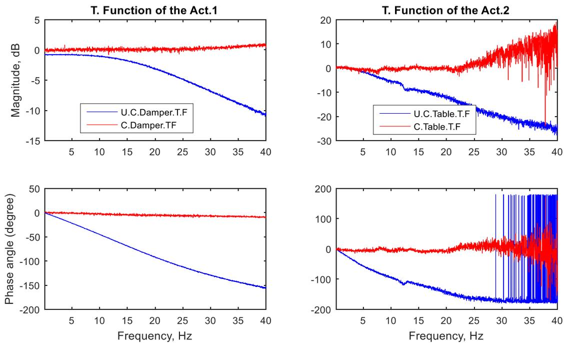
Fig. 5 Compensated and uncompensated Frequency response function of the actuators
