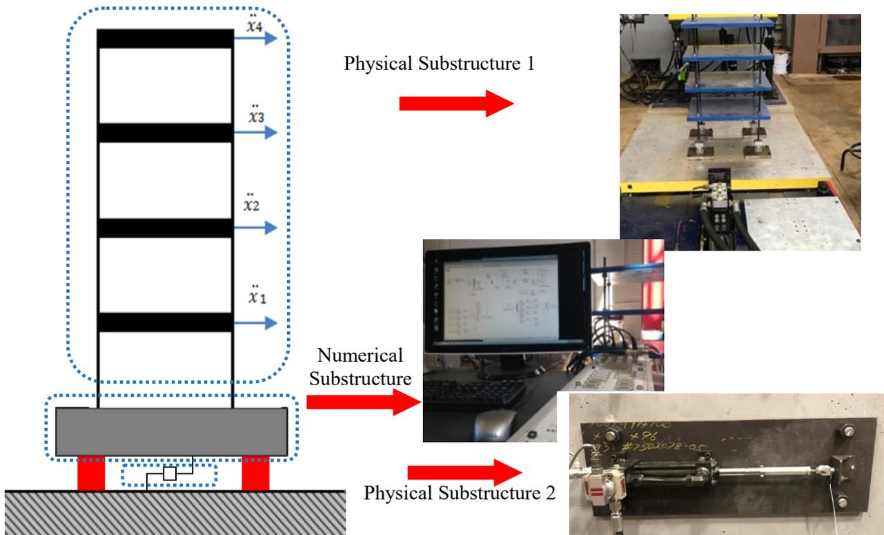
Fig.2 RTHS test configuration of a base isolated four story building structure
