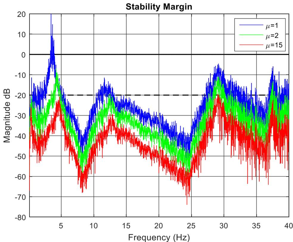
Fig. 6 Robust stability and performance margins of base isolated structure with a supplemental damper
