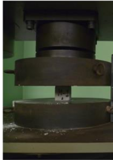
Fig. 4 - Compression test in mortar
