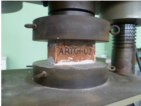
Fig. 3 - Compression test in bricks.
