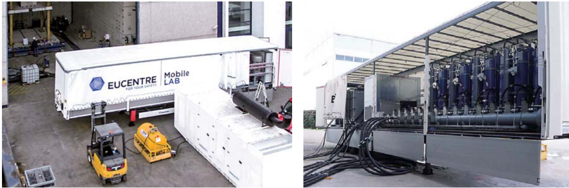
Fig. 1 – Overview of main trailer, pump, power station (left) and detail of the accumulators installed on the main trailer (right)
