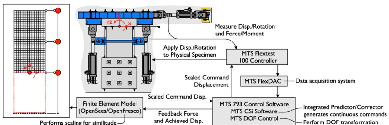
Fig. 4 – Hybrid test architecture
