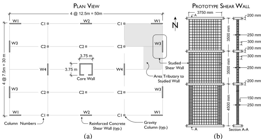
Fig. 1 – Three-storey prototype shear wall building: (a) floor plan; (b) typical shear wall detail
