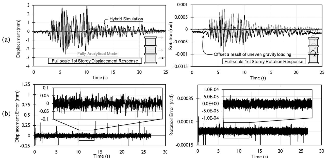
Fig. 6 – (a) Comparison of experimental and purely numerical displacement and rotation time-histories; (b) Displacement and rotation errors (difference between command and feedback for hybrid test)
