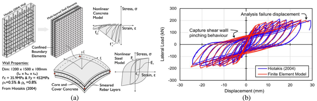
Fig. 9 – (a) Nonlinear multi-layer shell element; (b) Force-displacement hysteretic response comparison of nonlinear shear wall model with experimental results from Hiotakis (2004) [11]
