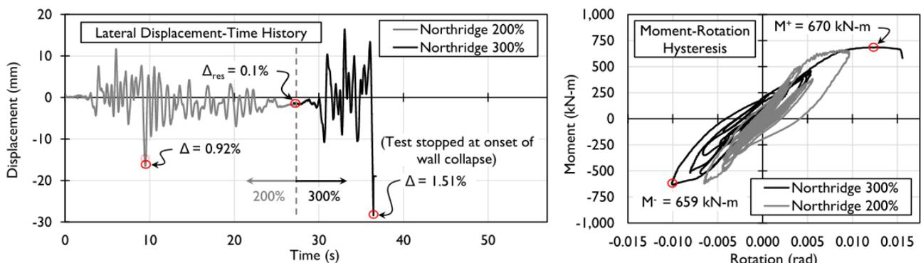
Fig. 7 – Displacement-time history and moment-rotation response for Northridge 200% and 300%
