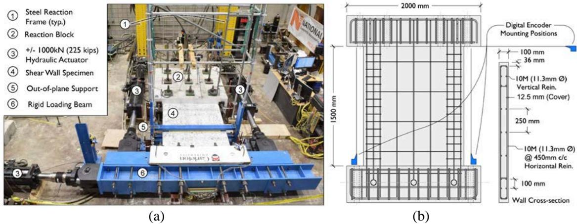
Fig. 3 – (a) Physically tested shear wall; (b) experimental test setup and encoder placement
