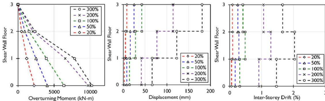
Fig. 8 – Global distribution of overturning moment, lateral displacement and inter-storey drift
