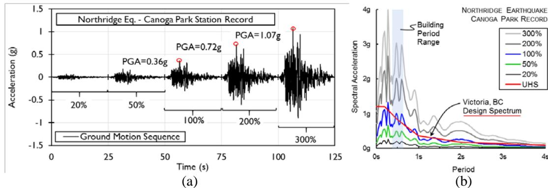
Fig. 5 – (a) Hybrid simulation earthquake sequence; (b) response spectra for the earthquake record set
