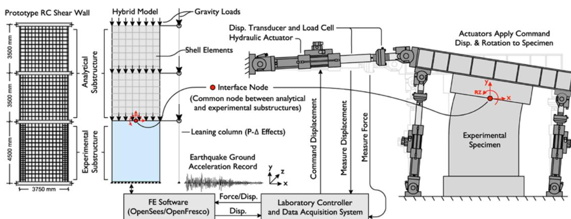
Fig. 2 – Hybrid simulation substructuring approach for multi-storey RC shear wall
