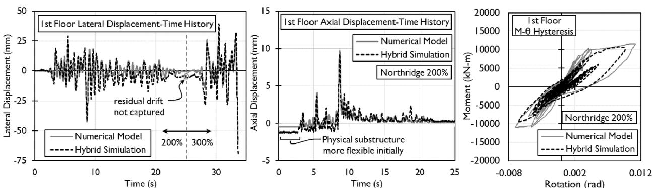
Fig. 10 – Comparison between hybrid simulation and purely numerical results for Northridge 200/300%
