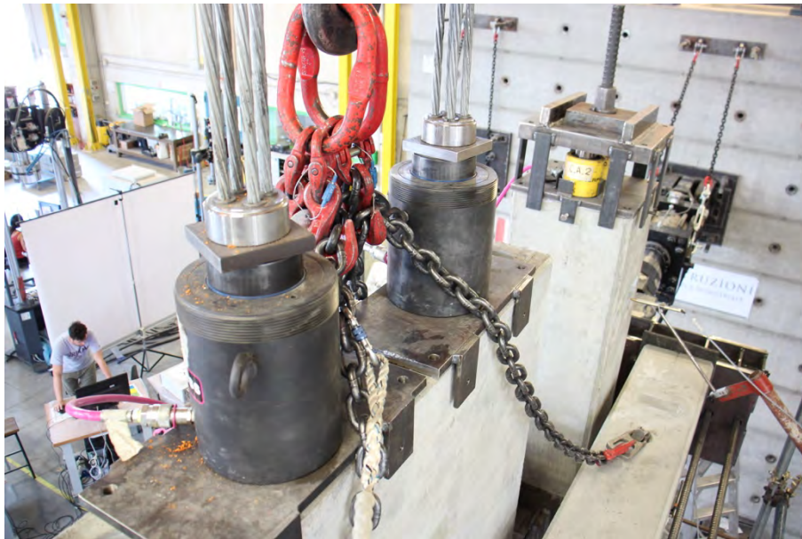
Fig. 5 – Hydraulic jacks at the top of the wall, used to measure the load on the cables.
