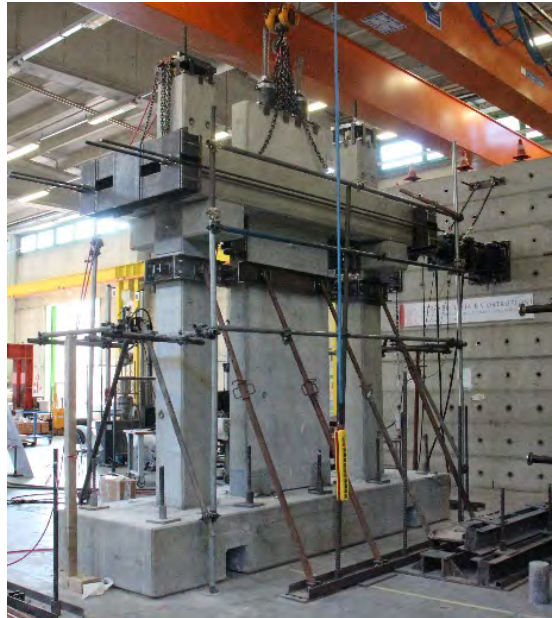
Fig. 1 – One of the structural systems tested under quasi-static lateral loads.
