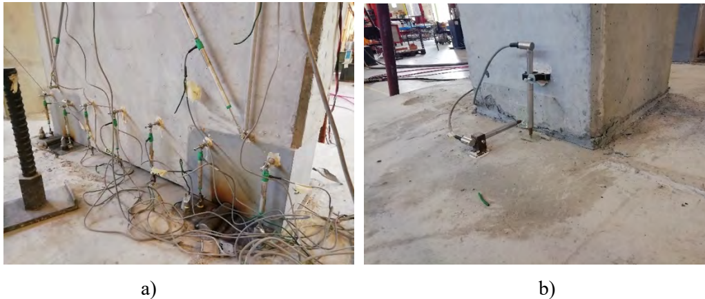
Fig. 4 – Displacement transducers at the base of the wall (a) and at the base of one of the two columns (b).
