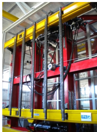
Fig. 3 – Test setup for connection of the cladding system to the testing machine.
