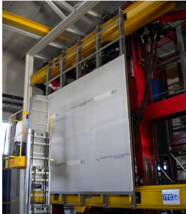
Fig. 6 – Assembly of the panels on zinc-coated aluminium framing system.
