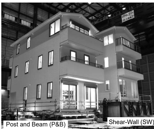
Fig. 1 – Test specimens were 3-story wooden houses.
