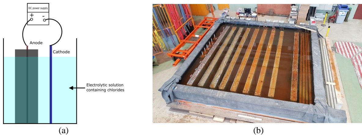
Fig. 2 – Accelerated corrosion technique. (a) Principle of the set-up, (b) Corrosion of the campaign beams
